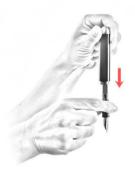
6. Screw the pen section back into the barrel.
